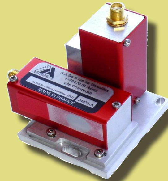
These deflectors offer a typical total resolution of 160 000 dots (2 axis) with a round input laser beam up to 6.7 mm ( $1/e^2$ ). Main advantage is the large scan angle which can reach up to 3 x 3 degrees.
